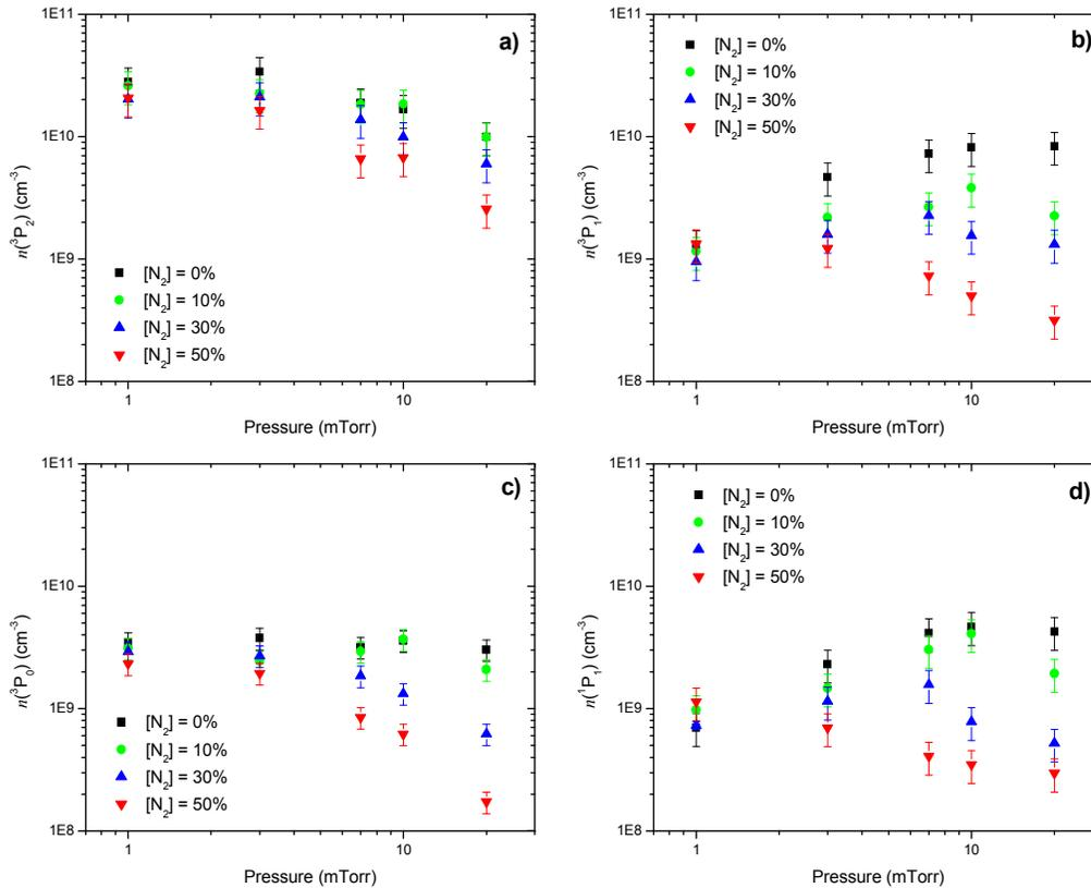
Fig. 1: Variation of the argon metastable ((a):  $^3P_2$ ; (c):  $^3P_0$ ) and resonant ((b):  $^3P_1$ ; (d):  $^1P_1$ ) densities with pressure for different nitrogen concentration.
