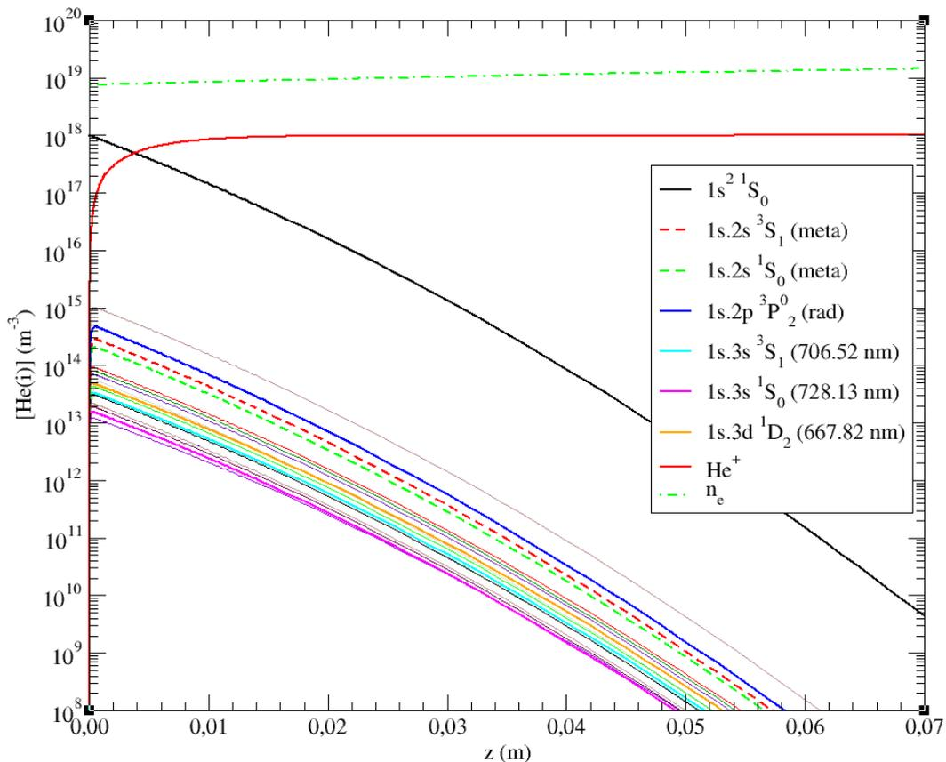
Fig.1. He excited states distribution in a typical edge plasma ( $dn_e/dx = 10^{20} \text{ m}^{-4}$  and  $dT_e/dx = 3 \times 10^7 \text{ Km}^{-1}$ ).
