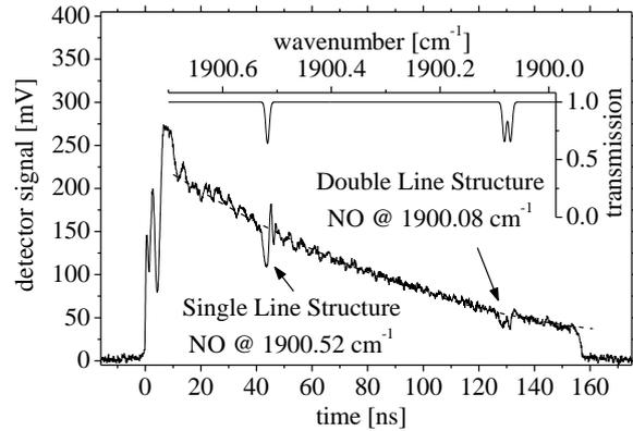
Fig. 2: NO spectrum (bottom) measured by QCLAS and a simulated spectrum (embedded diagram) using the HITRAN database [3] both for a gas mixture of 1% NO diluted in N<sub>2</sub> [1].
