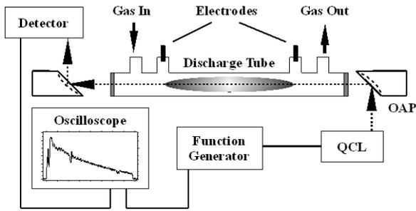
Fig. 1: Sketch of the experimental setup. The IR radiation passed the tube reactor three times. The T-shaped electrode holders allow spectroscopic studies in the homogenous part of the dc plasma [1].
