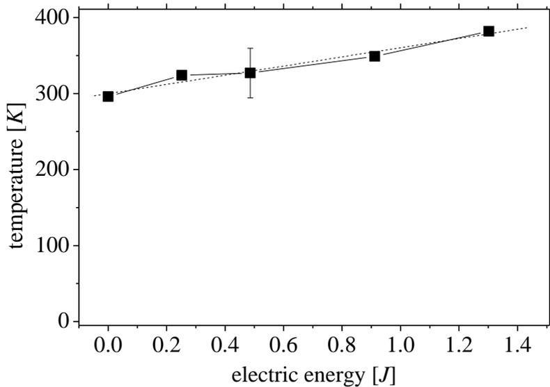
Fig. 3: Final NO temperature of a pulsed dc plasma measured using the line ratio method. The electric energy corresponds to a mean pulse current of 25mA, 50mA, 100mA and 150mA, respectively. The dashed curve shows a linear fit.
