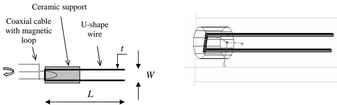
Fig. 1: a) Schematic view of the hairpin resonator wire with length  $L$  and cylindrical ceramic support; b) 3D model of the resonator, used in the Ansoft® HFSS simulator
