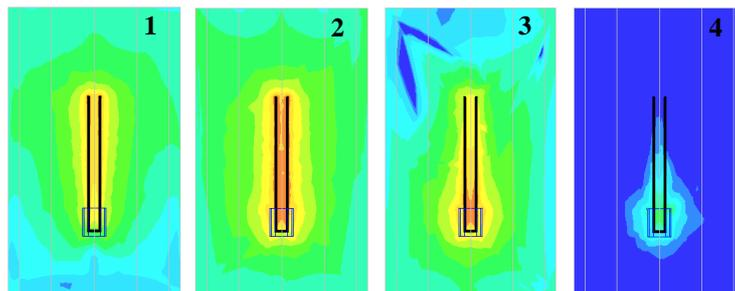
Fig. 4: Pictures of the simulated E field around the hairpin resonator in plasma with increased density (points 1, 2, 3 and 4 on Fig. 3).
