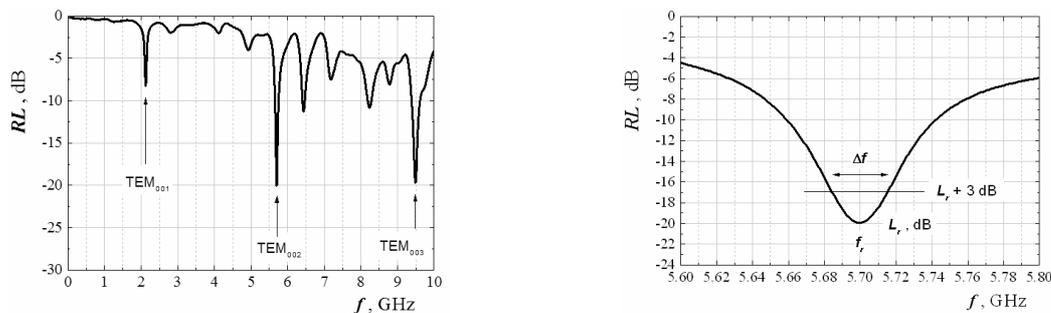
Fig. 2: a) Wide-band reflection response of the hairpin structure with the first three excited TEM resonances; b) Narrow-band response of  $TEM_{002}$  mode:  $f_{hairpin} \sim 5700$  MHz,  $\Delta f \sim 30$  MHz, loaded and unloaded Q-factors:  $Q_L \sim 190$ ,  $Q_0 \sim 211$
