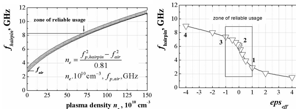
Fig. 3: a) Dependence of the hairpin resonance frequency v/s the plasma density; b) dependence of the resonance frequency v/s the effective plasma permittivity and simulated E-field distributions in 4 different points
