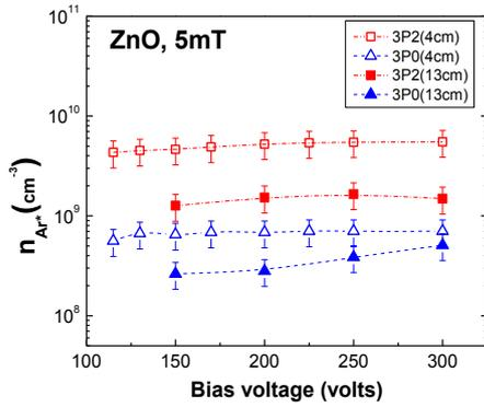
**Fig. 1:** Influence of the self-bias voltage on the number densities of Ar atoms in metastable  $^3P_2$  and  $^3P_0$  states at 4 and 13 cm from the ZnO target.
