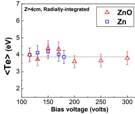
**Fig. 2:** Influence of the self-bias voltage on the radially-integrated electron temperature at 4cm from Zn and ZnO targets.
