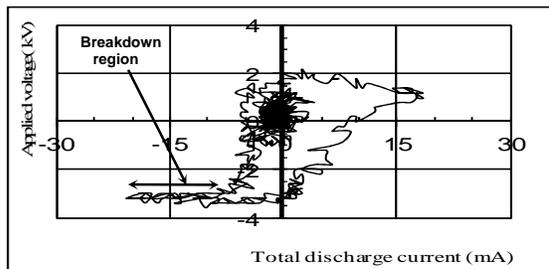
Figure 2: Lissajous V-I applied voltage on total discharge current
