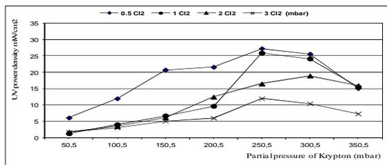
Figure 3: UV irradiance with partial pressure Krypton and chlorine at frequency of 100 kHz and width of 1.0 μs, taken on the excilamp wall.
