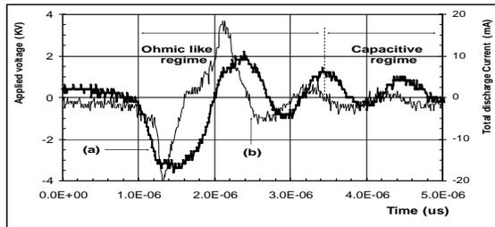
Figure 1: Typical waveforms of the voltage (a), current pulses (b), at 120KHz and 1.0us of width.
