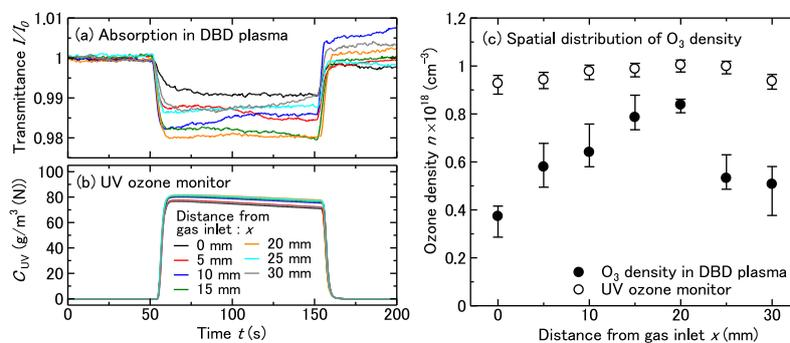
Fig. 2: Temporal variation of (a) transmittance and (b) ozone concentration by UV monitor. (c) Spatial distribution of ozone density in ozone reactor.
