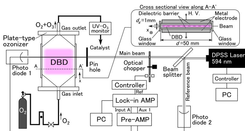
Fig. 1: Experimental setup for ozone density measurement.
