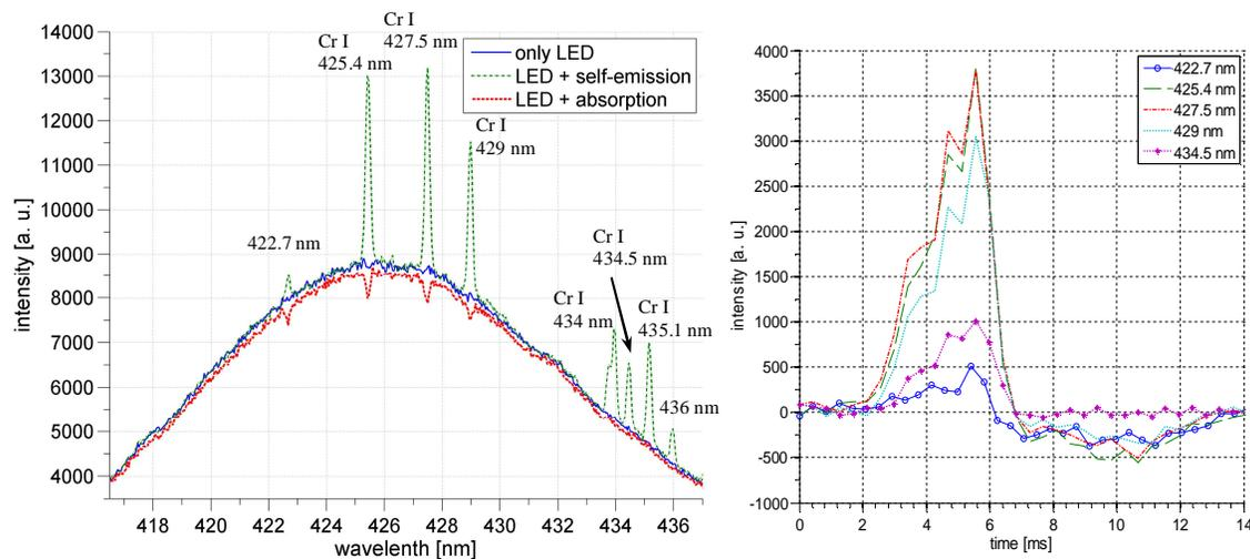
Fig. 2: Left) Three distinct cases of optical spectra: solid line shows only LED light at  $t = 0$  ms; in dash-dotted line the self-emission of the plasma at 5.8 ms is shown; dashed line corresponds to the absorption spectrum at 9.5 ms (2.5 ms after CZ). Right) Temporal evolution of the measured main relative spectral peak intensities (emission and later absorption).
