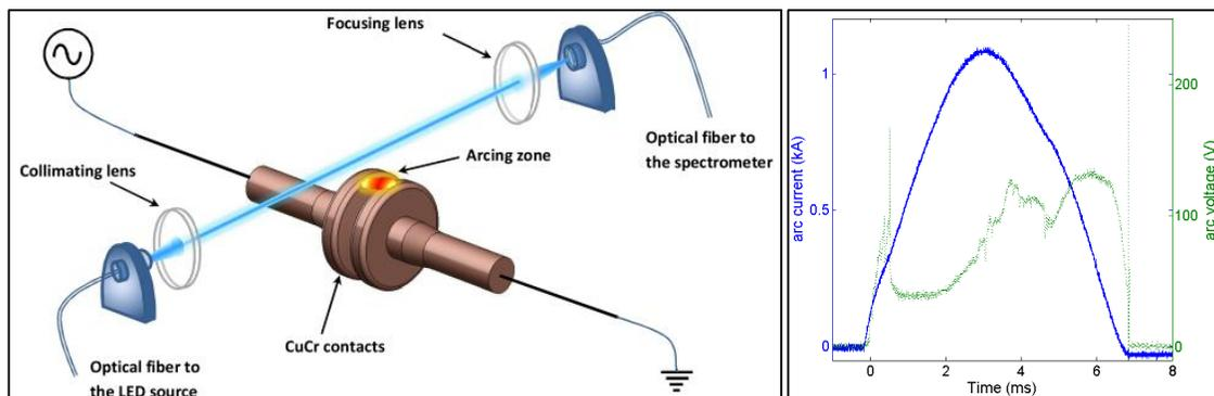
Fig. 1: Left: our experimental setup; Right: representative arc current and voltage recordings
