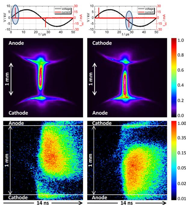
Fig. 1: ICCD pictures and streak images in both half-periods (indicated on top) of a sinusoidal driven DBD with  $U_{pp} = 14$  kV and  $f = 20$  kHz for 0.1 Vol.-%  $O_2$  in  $N_2$  in pseudocolor intensity scale.
