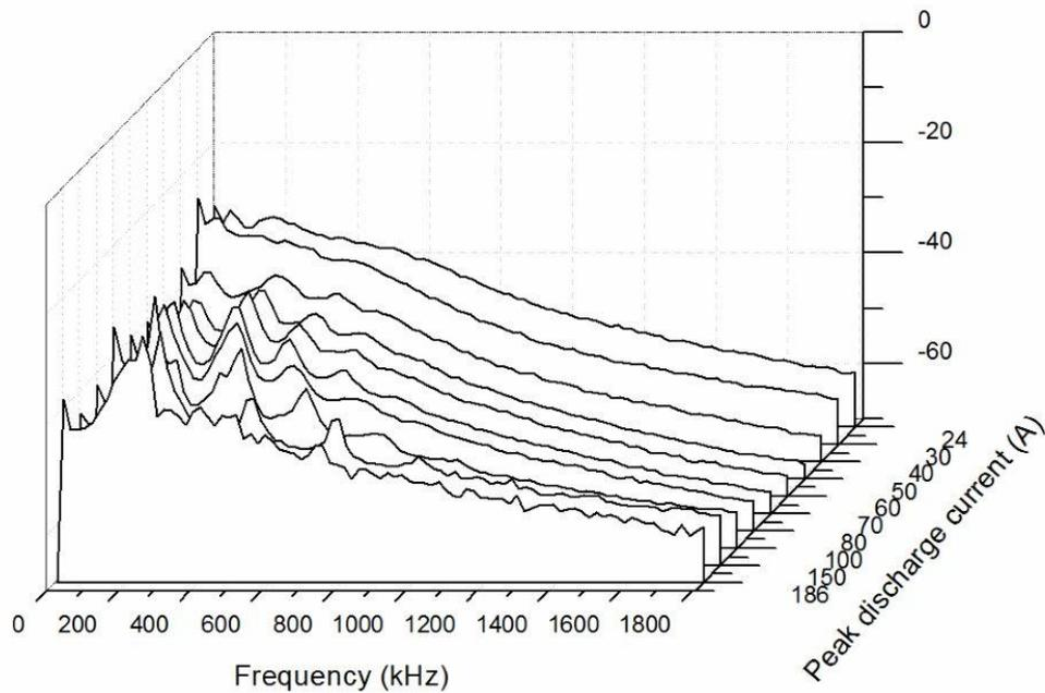
Fig. 2: FFT analysis of the frequency spectrum during a full discharge for different discharge currents (peak currents).
