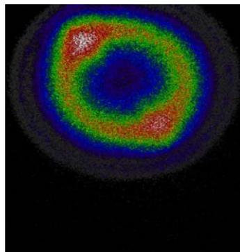
Fig. 1 : CCD image (frontal view) of the total light emission from the HPPMS discharge, showing an azimuthal mode number of  $m=2$ . Camera acquisition time: 150 ns
