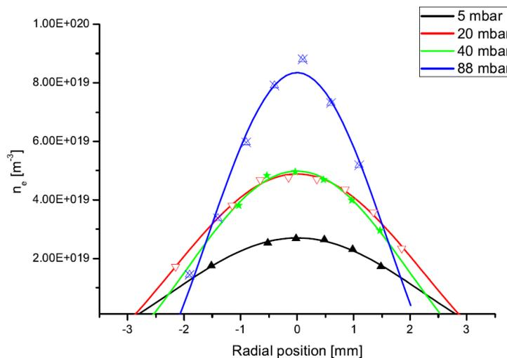
Fig. 1: Radial distribution of  $n_e$  with a Bessel function fitting in a surfatron argon plasma at various pressures. The inner tube radius is  $R=3$  mm.
