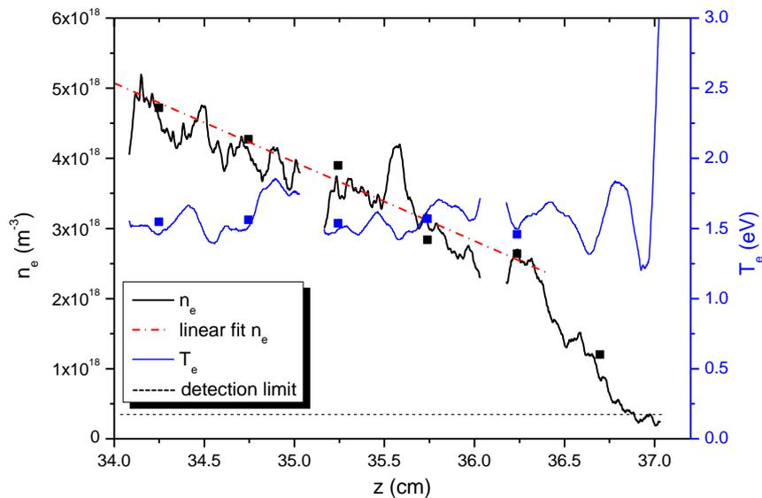
Fig. 2: The  $n_e$  and  $T_e$  values for 11 mbar obtained at the plasma column end with 3 frames of the iCCD. The symbols are Raman-calibrated TS results with pixel binning, while the curve presents the adjusted raw data. Note the steep drop of  $n_e$  in the very last frame, while  $T_e$  stays more or less constant at about 1.5 eV. At lower  $n_e$  values the low S/N ratio leads to very high (unphysical) values of  $T_e$ .
