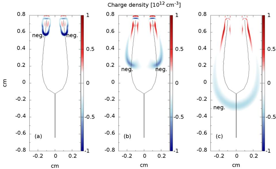
Fig. 1: Snapshots of different phases of evolution of the net charge density of two adjacent negative discharge filaments at ground pressure in air (sign of the charge in the discharge front is labeled), (a) 3.0 ns: two well developed streamers are repulsing each other, (b) 5.0 ns: the moment of transition between repulsion and merging, (c) 6.0 ns: after merging the discharge propagates through a single channel. Black solid line: complete trajectory of the maximum electric field.
