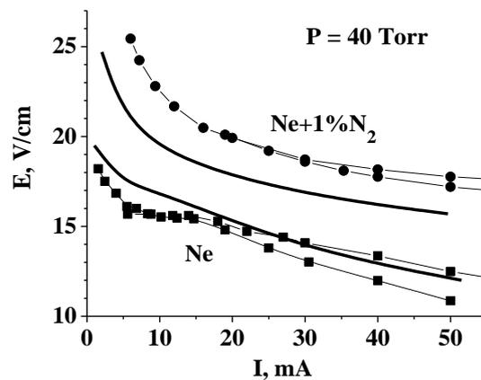
Fig. 2: Measured (symbols) and calculated (thick lines) dependences of the electric field in the positive columns of discharges in pure neon and the Ne + 1%  $N_2$  mixture on the discharge current for  $P = 40$  Torr.
