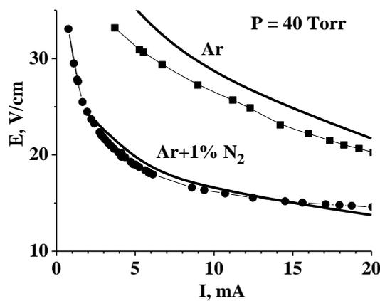
Fig. 1: Measured (symbols) and calculated (thick lines) dependences of the electric field in the positive columns of discharges in pure argon and the Ar + 1%  $N_2$  mixture on the discharge current for  $P = 40$  Torr [1].
