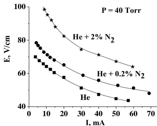
Fig. 3: Measured dependences of the electric field in the positive columns of discharges in pure helium and the He :  $N_2$  mixtures on the discharge current for  $P = 40$  Torr .
