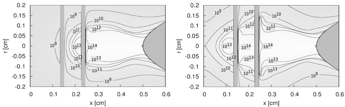
Fig. 1: 2D isocontours of the electron density at  $t=4.0$  ns (left) and  $t=5.7$  ns (right). Contours vary from  $10^9$  to  $10^{14}$   $\text{cm}^{-3}$ . Both dielectric planes have a thickness of  $176\mu\text{m}$  and a relative permittivity of  $\epsilon_r = 5$
