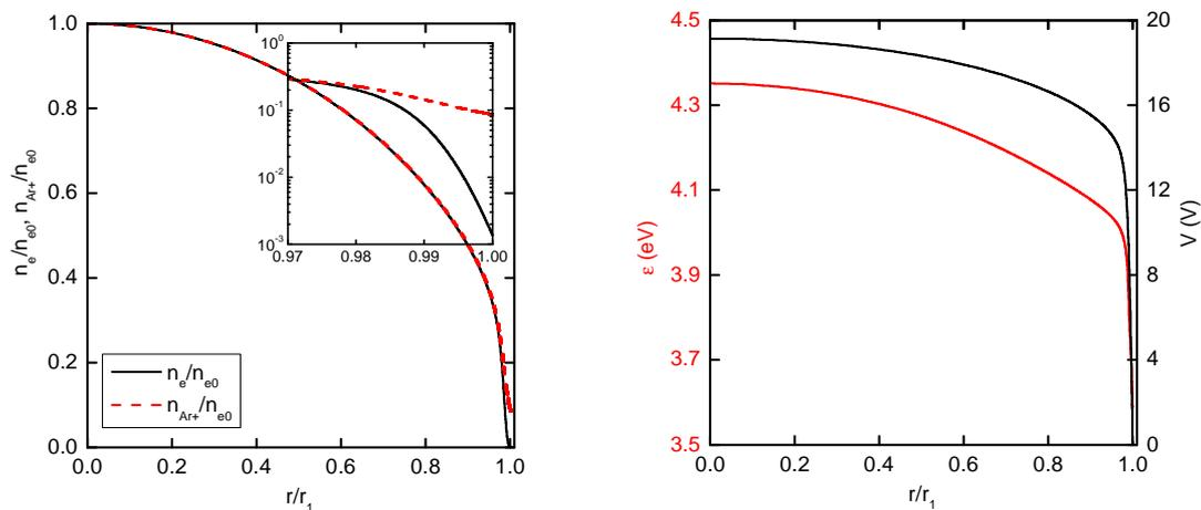
Fig. 2: Radial profiles, as a function of the normalized radius  $r/r_1$ , of the following quantities: left, the charged particle densities (electrons, solid curve; ions, dashed curve). The inset is just a zoom of this figure over the space-charge sheath region; right, the electron mean energy (red curve) and the plasma potential (black). Typical results obtained for  $r_1 = 50 \mu\text{m}$ ,  $n_e = 1.2 \times 10^{16} \text{ cm}^{-3}$ ,  $p = 0.1$  bar and  $T_g = 1000$  K.
