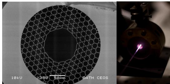
Fig. 1: Example of the cross-section of the HCPCF used during experiments (left) and image of the Ar micro-plasma created (right).
