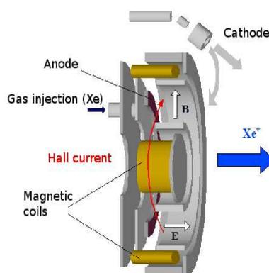
Fig. 1: schematic view of a HET.
