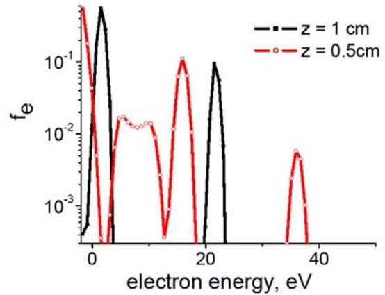
Fig.4: Electron energy distribution function on axis of symmetry at  $z=1$  cm (bulk plasma) and  $z=0.5$  (inside diaphragm hole)
