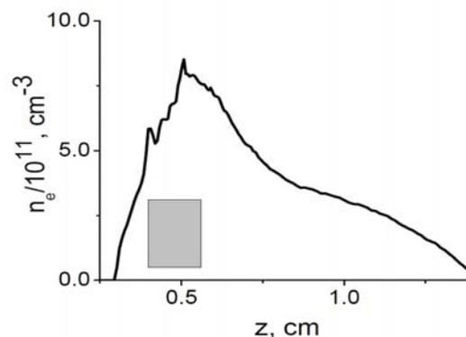
Fig. 2: Electron density profile along axis of symmetry. Grey box indicates location of the diaphragm.
