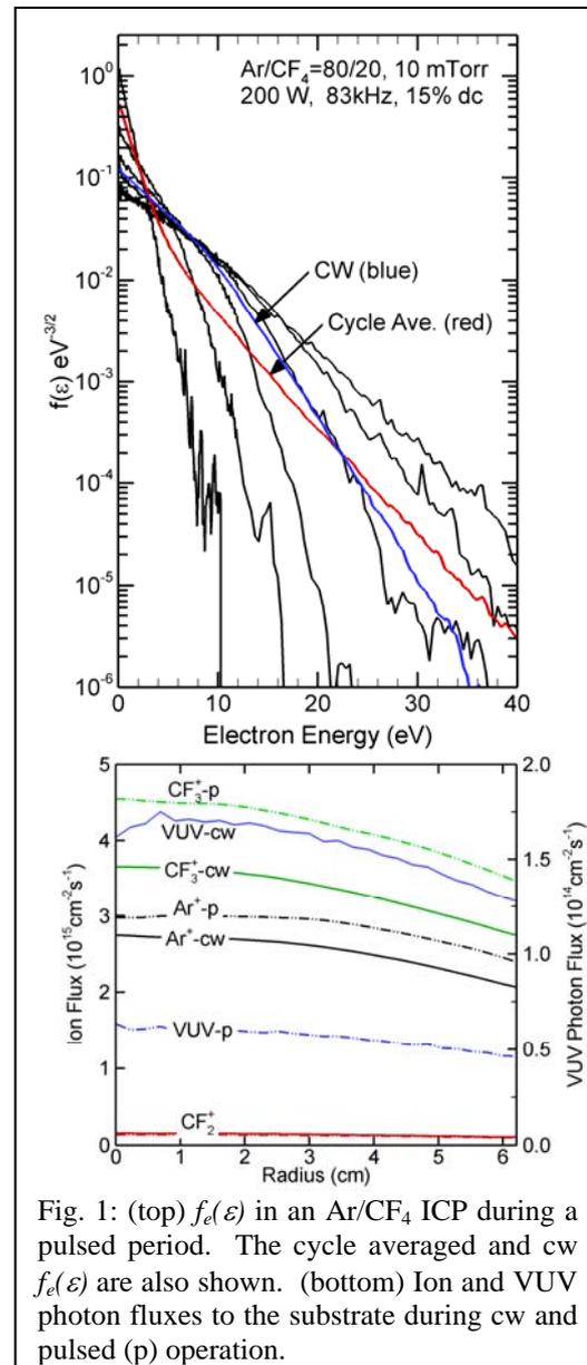
Fig. 1: (top)  $f_e(\epsilon)$  in an Ar/CF<sub>4</sub> ICP during a pulsed period. The cycle averaged and cw  $f_e(\epsilon)$  are also shown. (bottom) Ion and VUV photon fluxes to the substrate during cw and pulsed (p) operation.
