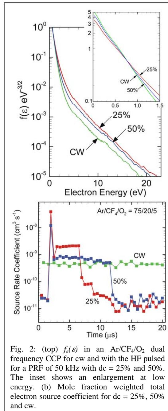
Fig. 2: (top)  $f_e(\varepsilon)$  in an  $\text{Ar}/\text{CF}_4/\text{O}_2$  dual frequency CCP for cw and with the HF pulsed for a PRF of 50 kHz with dc = 25% and 50%. The inset shows an enlargement at low energy. (b) Mole fraction weighted total electron source coefficient for dc = 25%, 50% and cw.
