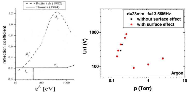
Fig. 2: Figure from the left side presents coefficient of reflection and emission of secondary electrons from surface of electrode made of steel [9] (our input data). Figure on the right side is Paschen curves with and without surface effect included.
