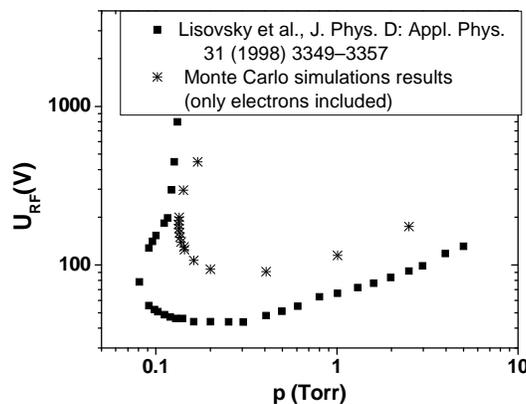
Fig. 1: Paschen curve for rf breakdown in argon, at 13.56 MHz and gap size 23mm, comparison of experimental and MC simulation results
