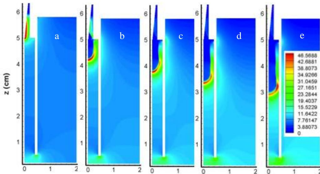
Fig. 2: Spatial distribution of reduced electric field (Townsend) at different times t. Figure a: t=0, Figure b: t=56 ns, Figure c: t=116 ns, Figure d: t=176 ns, Figure e: t=236 ns.
