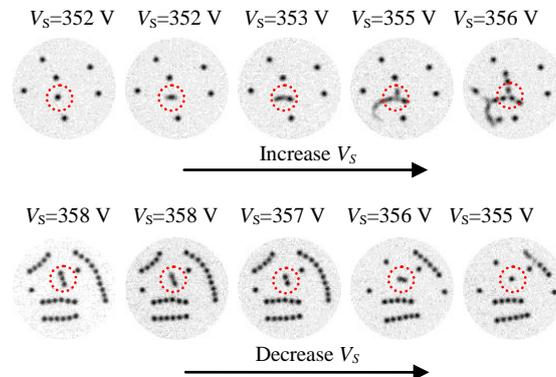
Fig. 2: The process of splitting of a single filament (the upper, increasing voltage) and quenching of filaments (the bottom, decreasing voltage) at  $p = 30$  Torr and  $f = 50$  kHz.
