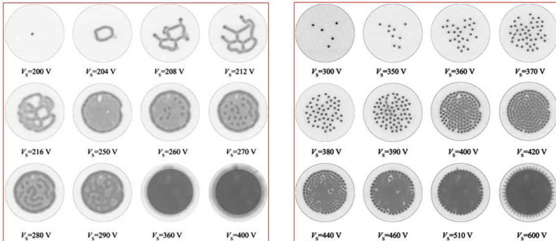
Fig. 1: The images of the DBD pattern from top-view at increasing voltages for (a) the left:  $p = 7.5$  Torr,  $f = 20$  kHz and (b) the right:  $p = 30$  Torr,  $f = 50$  kHz. The exposure time is 1 s.
