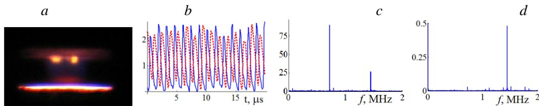
Fig. 2. Image of two anode spots (*a*), their light intensity waveforms (*b*) and Fourier-spectra of the spot intensity (*c*) and discharge current (*d*) oscillations. Vertical scales – arbitrary units.
