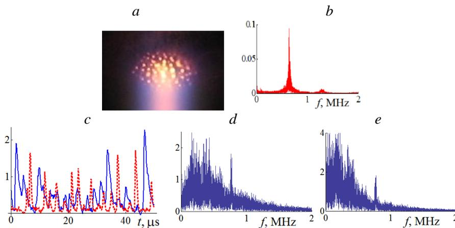
Fig. 3. Image of anode spots pattern (*a*), Fourier-spectrum of current oscillation (*b*), light intensity waveforms (*c*) and their corresponding Fourier-spectra (*d*) and (*e*). Vertical scales – arbitrary units.
