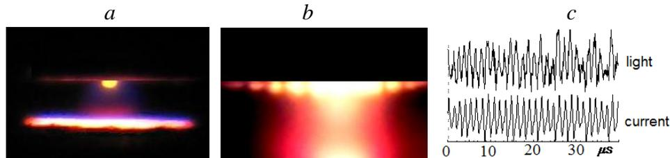
Fig. 1. Images of the anode spots at different interelectrode gaps and discharge currents: *a* – less than 1 mm and 10 mA, *b* – 8 mm and 200 mA. Waveforms of the current and light oscillation (*c*).
