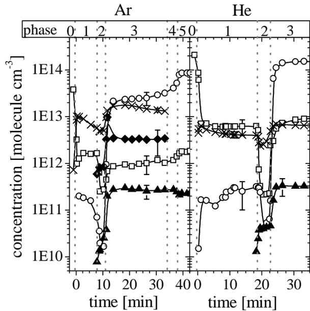
Fig. 1: Molecular concentrations in Ar, left panel, and He RF plasmas, right panel, with admixtures of  $C_2H_2$  or  $CH_4$  in different experimental phases, as a function of the time ( $\square$  -  $C_2H_2$ ,  $\circ$  -  $CH_4$ ,  $\blacklozenge$  -  $C_2H_4$ ,  $\blacktriangle$  -  $CH_3$ ,  $\times$  -  $CO$ ).
