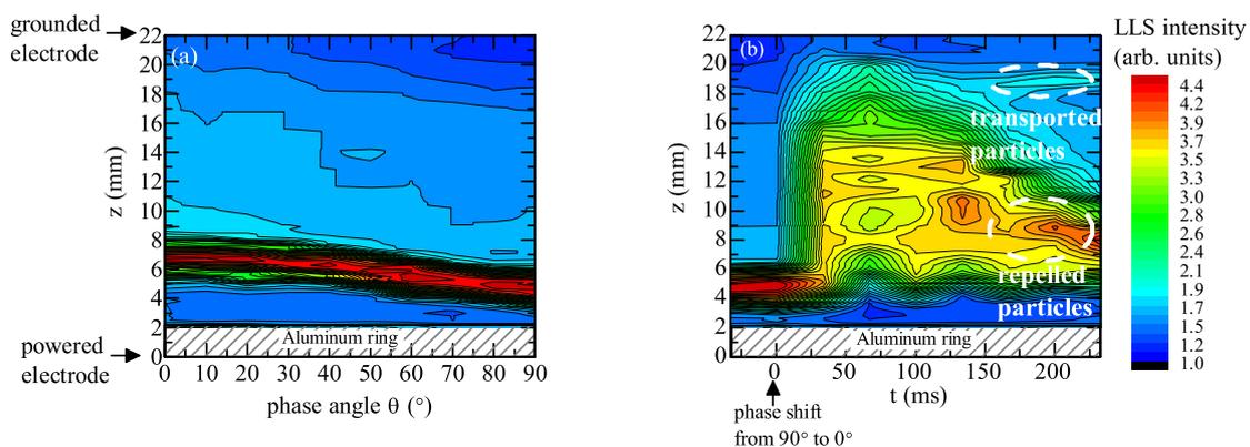
Fig. 1: (a) Spatiotemporal profile of the laser light scattering (LLS) intensity from the dust particles obtained by the (a) adiabatic or (b) sudden phase shift from  $90^\circ$  to  $0^\circ$  for  $\phi_0 = 100$  V and  $p = 2$  Pa.
