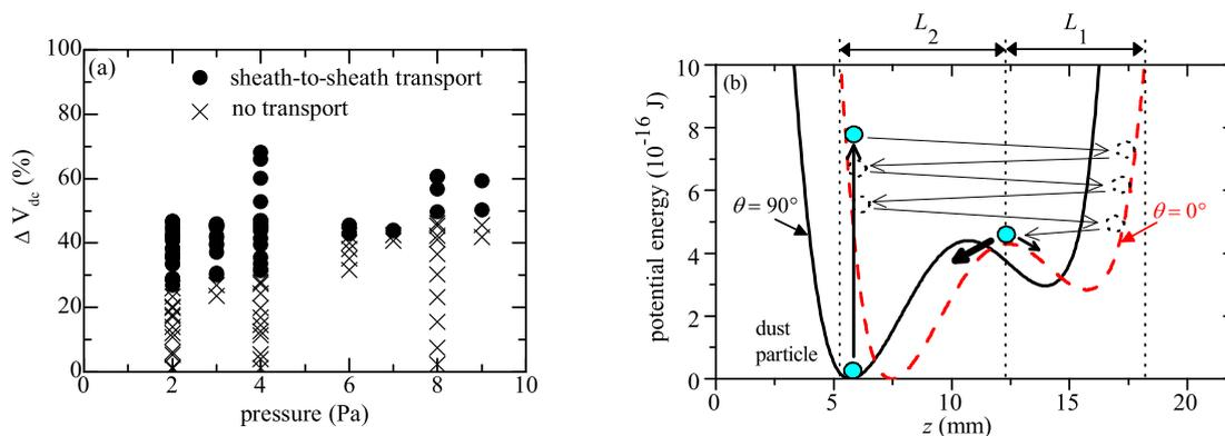
Fig. 2: (a) Classification of the sheath-to-sheath transport as parameters of pressure and change of self bias  $\Delta V_{dc}$ . (b) Spatial profiles of the potential energy calculated from PIC simulation data for  $\theta = 0^\circ$  and  $90^\circ$ .
