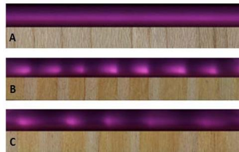
Figure 1: Spatial distribution of the He plasma in presence of a sugar maple substrate (A) and Douglas pine samples with tight (B) and wide (C) late and early wood sections.
