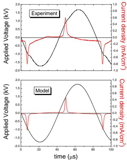
Figure 2: Measured and simulated I-V characteristics for a pure He plasma in presence of a Douglas pine sample. Applied voltage : 3.5 kV<sub>pk-pk</sub> at 12 kHz.
