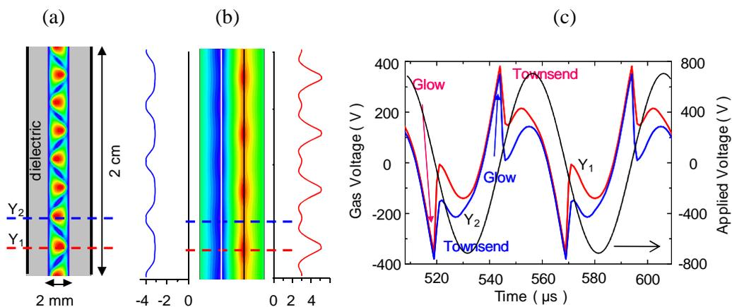
Fig. 4: Quincunx structure predicted by the model. (a) Electron density integrated over one period (log scale on two decades with max =  $4 \cdot 10^9 \text{ cm}^{-3}$ ); (b) distribution of surface charges on left and right dielectrics and potential distribution just before a current pulse (max in red = 212 V and min in purple = -182 V); (c) gas and applied voltages. Conditions are: Neon gaz at 50 torr,  $V_m = 700 \text{ V}$ ,  $f = 20 \text{ kHz}$ .
