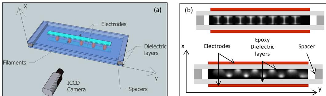
Fig. 2: 1D self-organized patterns of filaments. (a) Sketch of the 1D geometry, filament patterns are observed through a transparent electrode along the discharge axis  $x$  or along the direction of pattern formation  $y$ ; (b) on top the classical filamentary discharge and on bottom the quincunx structure (Neon gaz at 50 torr,  $V_m = 524$  V,  $f = 30$  kHz).
