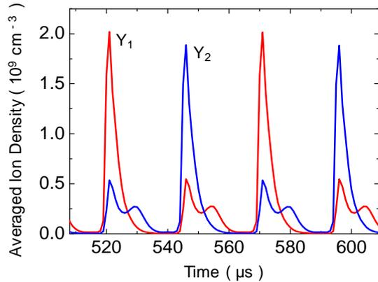
Fig. 5: Averaged ion density along  $x$  axis as a function of time for two  $y$  positions.  $Y_1$  in red corresponds to the bottom position in Fig. 4a and  $Y_2$  in blue to the top one. Conditions are the same as in Fig. 4.
