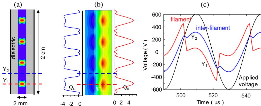
Fig. 3: Classical filamentary pattern predicted by the model. (a) Electron density integrated over one period (log scale on two decades with max =  $7.5 \cdot 10^9 \text{ cm}^{-3}$ ); (b) distribution of surface charges on left and right dielectrics and potential distribution just before a current pulse (max in red = 325 V and min in purple = -112 V); (c) gas and applied voltages. Conditions are: Neon gaz at 50 torr,  $V_m = 600 \text{ V}$ ,  $f = 25 \text{ kHz}$ .
