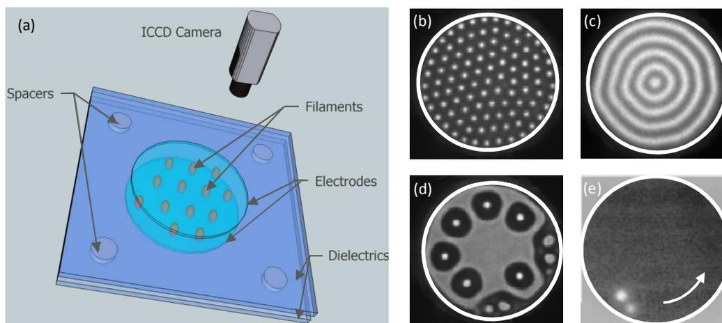
Fig. 1: 2D self-organized patterns of filaments. (a) Sketch of the 2D geometry, filament patterns are observed through a transparent electrode; (b) hexagonal; (c) target; (d) hybrid; (e) pair of filament in motion (from Ref. [4]). The conditions are: 2 mm gas gap filled with neon at pressure around 0.1 atm, between two 2mm glass dielectric layers covered with circular electrodes of 55.4 mm diameter and powered with sinusoidal voltage of 500-1000 V amplitude at frequency in the 10 kHz range.
