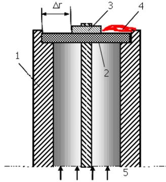
Fig.3. Scheme of “Microwave Arc”. 1-outer electrode; 2-quartz disk; 3-inner electrode; 4- discharge channels; 5-microwave radiation.
