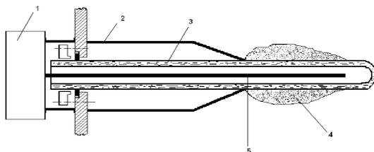
Fig.1. Schematic of coaxial microwave plasmatron 1-magnetron; 2-outer electrode; 3-quartz tube; 4-gas-discharge near-the-surface plasma layer; 5-inner electrode – rod; 6-wall of reactor chamber
