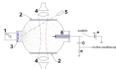
Fig.2. Scheme of experiment with the “biresonant” plasmatron. 1-cylindrical waveguide; 2-quartz window; 3-plasma-forming window; 4-horn-lens antennas of microwave interferometer; 5-plasma of “halo” optical spectrograph; 6-Langmuir probe.
