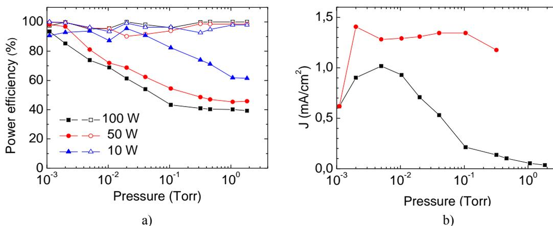
Fig. 2 a) Transmitted power efficiency as a function of pressure for three incident power values  $P_i = 10, 50$  and  $100$  W, with (empty symbols) and without (full symbols) impedance matching; b) Current density collected at 6 cm from the reactor wall as a function of pressure, when 100 W are fed in the plasma source, with (circles) and without (squares) impedance matching.
