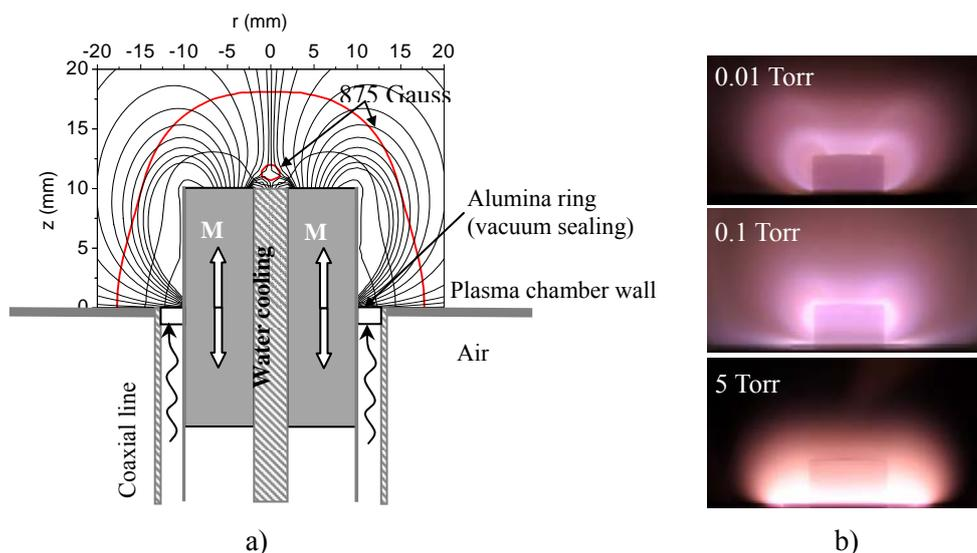
Fig. 1 a) Elementary plasma source based on coaxial transmission line ended by top-to-tail magnetic configuration; b) Pictures of argon plasma (30 W, 2.45 GHz) for three pressures.
