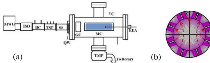
Figure 1 (a): Schematic of the experimental set-up: MWG, microwave generator; ISO, magnetron oscillator; DC, directional coupler; TST, triple-stub tuner; SS, straight section; QW, Quartz window; GC, guiding cylinder; VC, vacuum chamber; MC, multicusp; TMP, turbo molecular pump; EEA, electron energy analyzer or a Langmuir probe or an antenna probe (b) POISSON simulation showing the minimum B magnetic field with the electric field structure of the TE<sub>11</sub> mode superposed.
