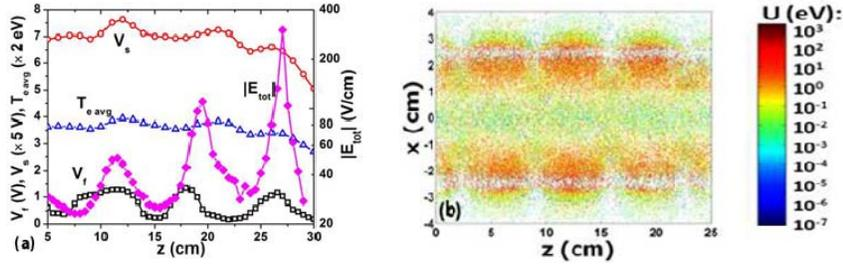
Figure 2 (a) Axial variation of calibrated  $|E_{tot}|$  (diamond),  $V_f$  (square),  $V_s$  (circle), and  $T_{e\_avg}$  (triangle) with 180 W power, at 0.25 mTorr pressure. (b) Simulation of electron energy in a section parallel to the MC axis.
