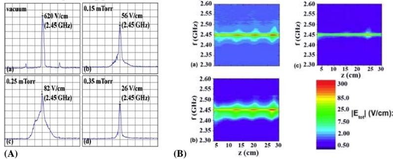
Figure 3: Wave spectrum screenshot at 180 W at different pressures and at  $z = 18$  cm. Central frequency = 2.45 GHz, and span = 300 MHz. (b) Asymmetric spectral broadening of central frequency (2.45 GHz) versus  $z$  at (a) 0.15 mTorr, (b) 0.25 mTorr, and (c) 0.35 mTorr, at 180 W.
