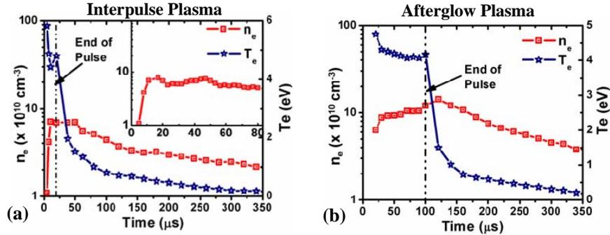
Figure 2: The  $n_e(t)$  and  $T_e(t)$  profile at (a) 20  $\mu\text{s}$  pulse duration with an inset showing an expanded view of  $n_e(t)$  indicating interpulse plasma, and at (c) 100  $\mu\text{s}$  indicating afterglow plasma.
