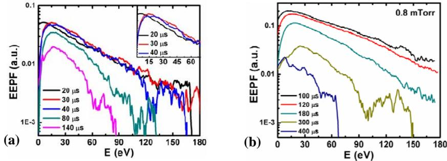
Figure 3: EEPF evolution after the end of the pulse for pulse duration (a) 20  $\mu\text{s}$ , and (b) 100  $\mu\text{s}$ .
