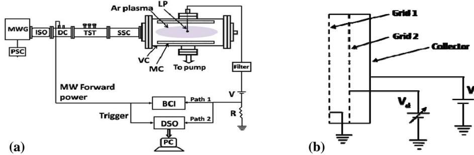
Figure 1 (a): Schematic of the experimental set-up: PSC, power supply and controller; MWG, microwave generator; ISO, magnetron oscillator; DC, directional coupler; TST, triple-stub tuner; SSC, straight section; VC, vacuum chamber; MC, multicusp; LP, Langmuir probe; BCI, box-car integrator; and DSO, digital oscilloscope, (b): Bias scheme of Electron Energy Analyzer EEA, which consists of two grids and a collector (spacing between each is 0.5 mm, diameter 3 mm).
