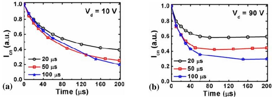
Figure 4: Temporal variation of EEA collector current after the end of the pulse (taken as  $t = 0$ ), as a function of microwave pulse duration, by keeping discriminator voltage at (a) 10V and, (b) 90V.
