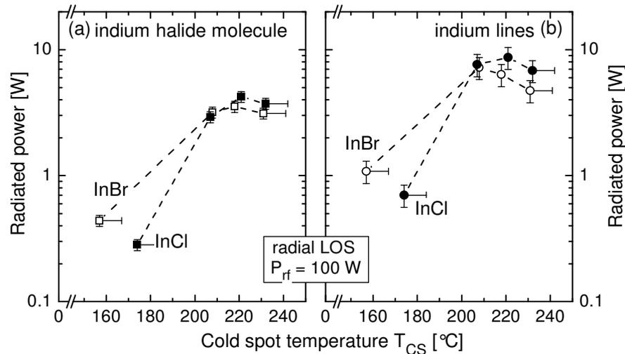
Fig. 2: Radiated power of the indium halide molecule (a) and the indium lines (b) in ICP discharges of InBr in argon and InCl in argon respectively, at a pressure of 1 mbar.
