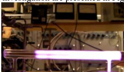
Fig. 1b: SWD between two dielectric tubes with metal antenna at the axis – coaxial configuration [2–4]
