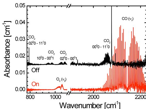
Fig. 3: FT-IR spectra recorded from the exhaust of a flow-tube DBD in  $\text{CO}_2$  for plasma-off (upper trace) and plasma-on (lower trace, differential spectrum) conditions. In the upper trace different vibrational transitions are labelled. The lower trace shows the main products: CO and  $\text{O}_3$ .
