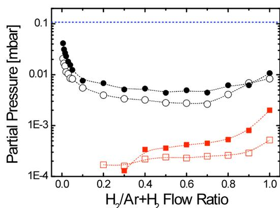
Fig. 2: CO (circles) and  $\text{CH}_4$  (squares) partial pressures measured in the expansion of an arc plasma created from Ar/ $\text{H}_2$  mixtures (full symbols). The initial  $\text{CO}_2$  concentration is indicated (dotted). Note the logarithmic scale.  $\text{CO}_2$  dissociation up to 50 % in Ar is detected. Using copper as wall material the CO concentration was significantly reduced and so was the  $\text{CH}_4$  production (open symbols).
