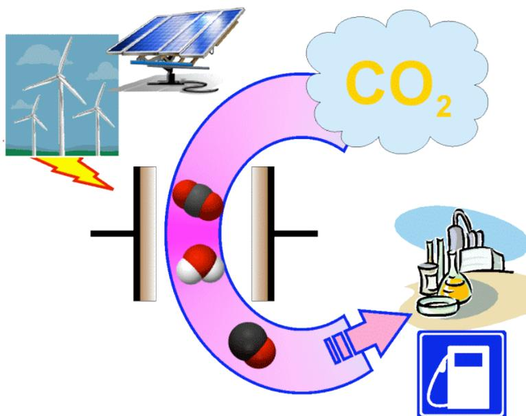
Fig. 1: Fuel processing in a closed-loop carbon cycle based on plasma-assisted CO<sub>2</sub> dissociation and hydrogenation assuming that electrical energy to drive the plasma source is provided from renewable sources.
